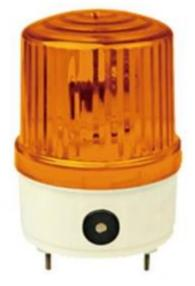
Easy to wear with low noise gear transmission mode, scientific parabolic mirror so that the light spread to far. Speed: 90-130RPM; Material: shade -AS, base -ABS, mirror -PC; protection class IP45; product with a buzzer, Volume: 85dB above; installation of: bolt-on; with high strength, able to adapt to harsh environments. Colors are red, yellow, green and blue
